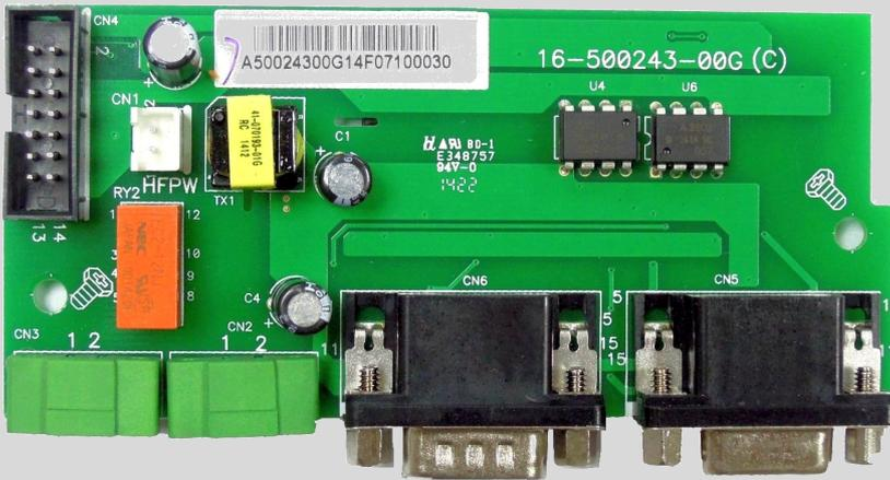
This accessory is applicable only to select 48VDC models of HS and MS series inverters. It is a required component to be installed in every unit of a parallel system. A parallel kit includes:
